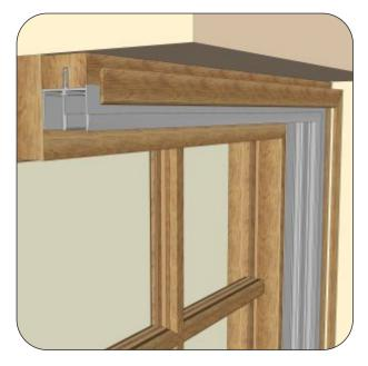
6 Cut and mitre beads to suit the frame. Using your own judgement obtain the best possible sight lines between frame and beads, these may not run 100% parallel and over lap metal depending on trueness of reveal. Attach trims in place using super glue or silicone.
