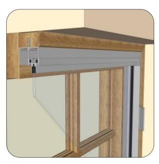
Apply the smallest possible acrylic seal between the reveal and the trim (size depends on trueness of reveals).
