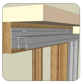
Screw directly into the existing window using the pre-drilled holes on the odd leg frame. (While fixing make sure secondary is level)
