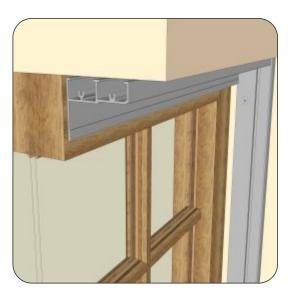
3 Locate the outer frame into the reveal in the position required and fix in place. Pack the frame as required to ensure it is installed square and true in every aspect.
