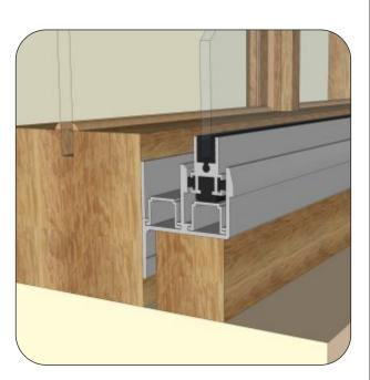
4 Note that packing could be required beneath the secondary frame to support the weight of the panels. This support will not be provide and will require your own judgment.
