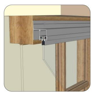
3 Insert each panel into the frame. Once assembled check that all panels work correctly. If not adjust where needed.
