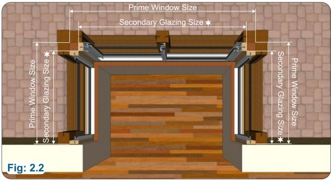
Fig 2.0 Shows a cut through of a square bay window with secondary installed.
