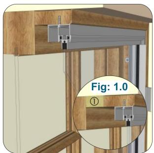
**8** Apply the smallest possible acrylic seal between the reveal and the trim (size depends on trueness of reveals).
