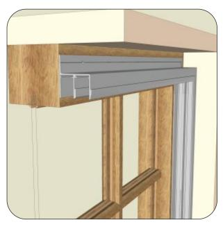
Locate secondary frame into aperture. Make sure secondary is level before moving onto fixing.
