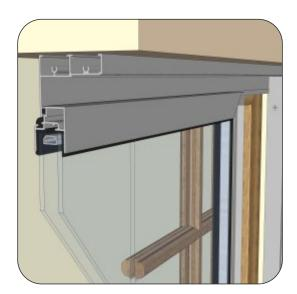
Insert correct panel into the back track of the cill and push into the vertical position and support it to prevent it falling forward (ensure interlock is facing into the room).
