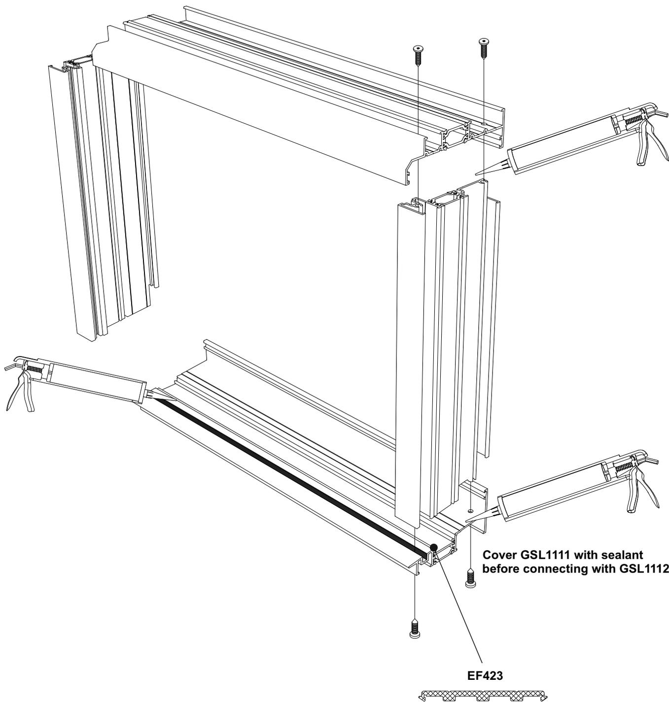
EF423 Will be inserted and sealed in the factory. This provides a water tight seal along the length of the threshold.
